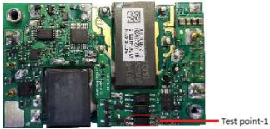
Figure 12 Temperature test points
