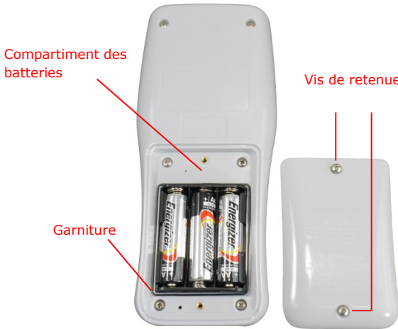
Figure 1: Installation des batteries
