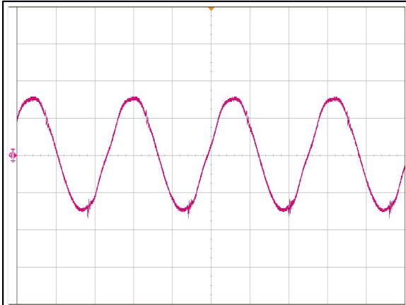
Figure 1: AVD85B-48S12 Input Reflected Ripple Current Waveform 1uS/div Ch 4: lin (20mA/div)
