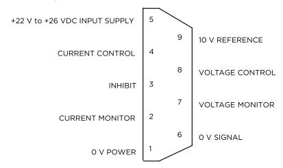
The above pinout diagram is view looking at the connector pins.
