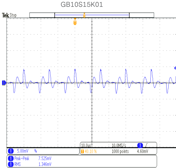
Figure 64: Common Mode Current at 115Vac Current Probe:1mA/mV
